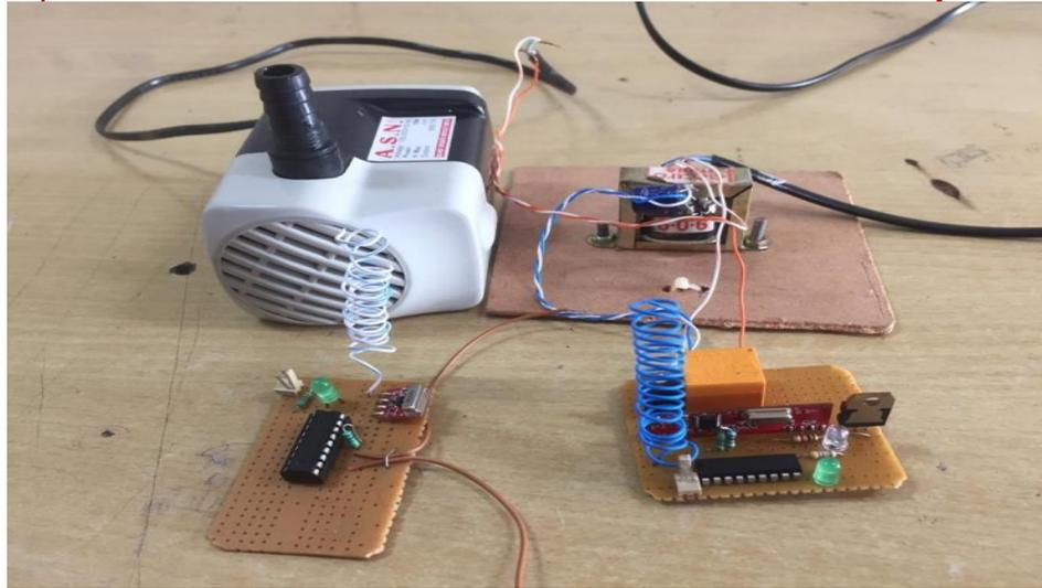
Figure 7: Implementation of the water detection system
