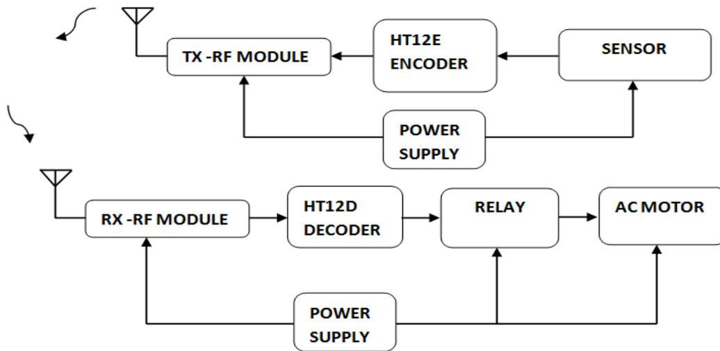
Figure 3: Block Diagram of automated water level controller
