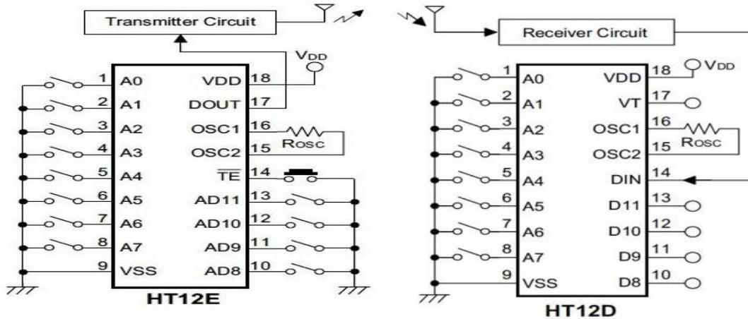
Figure 1: Pin diagram and connections of Encoder and Decoder
