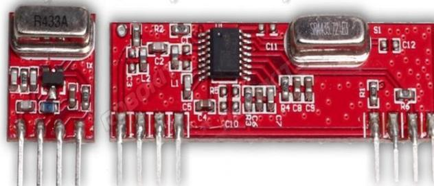
Figure 2: RF module of transmitter and receiver
