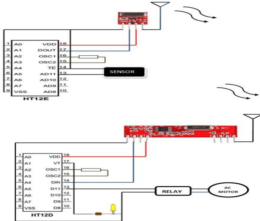
Figure 6: Circuit Diagram of the project
